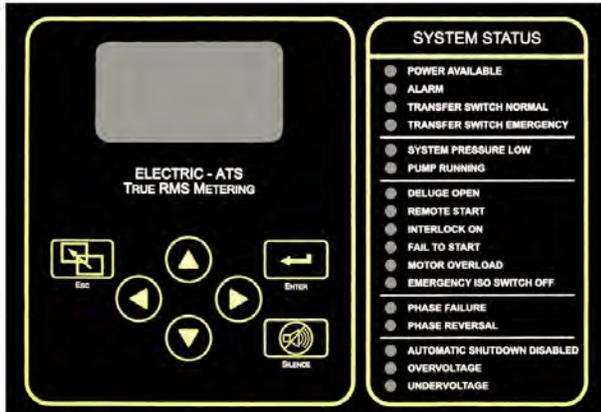
**Description**—Firetrol® FTA740 Single Phase Limited Service Controllers are intended for use with small electric motor driven fire pumps where the capacity of the power source permits full voltage starting. Full voltage is applied to the motor as soon as the controller is actuated. The controller monitors, displays and records fire pump system information.
